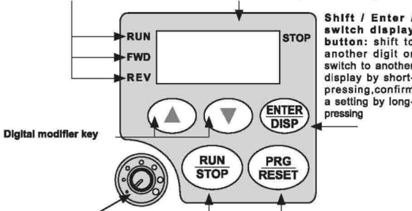
Turn to another frequency by rotating the potentiometer when the frequency is set to be controlled by the manipulator potentiometer
