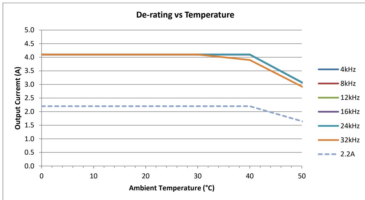
**7.3.2.5 Frame Size 2, IP66, 110 – 115V 1 Phase Input, 230V 3 Phase Output (Voltage Doubler), 5.8A**
