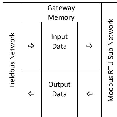
The fieldbus Master can normally be configured to Read and Write the entire gateway memory area in a single transaction, or separate transaction per drive may be configured. The gateway is the pre-configured by Invertek to carry out the necessary individual Modbus RTU transactions to communicate with the Sub Network of connected drives.
