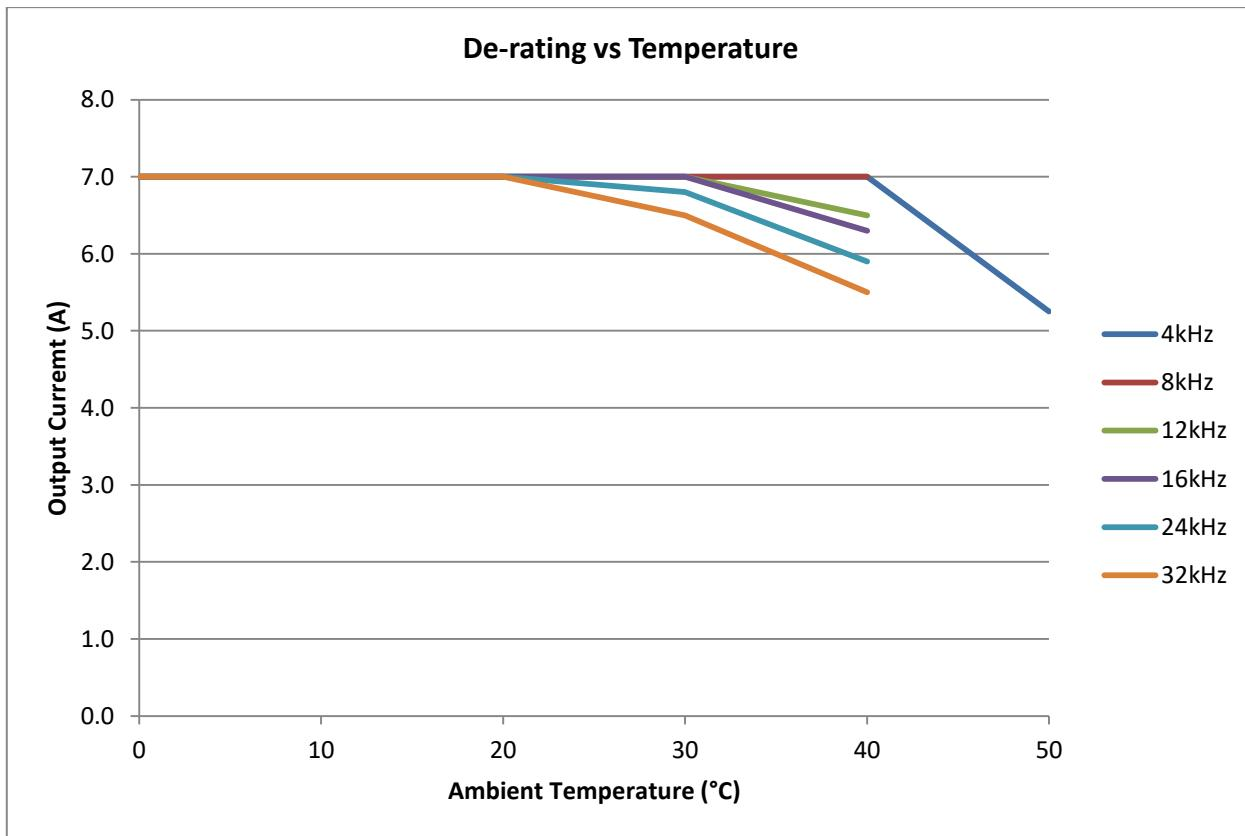
**7.3.4.2 Size 1, IP66, 200-240V 1Ph Input, 1Ph Output, 4.3A & 7A**
