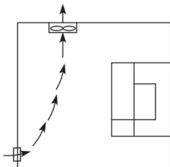
Correct installation position of the fan
